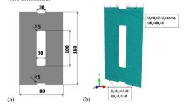
Figure 1: Plate with a notch: (a) dimensions in mm, (b) FE-model of the plate
