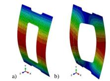
Figure 3: The buckling modes obtained using FEM (a) flexural buckling mode, (b) flexural-torsional buckling mode
