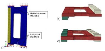
Figure 2: FE-model of the tested plate with fixed stripes
