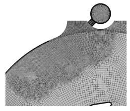
Figure 2. Discretization of the supply region
