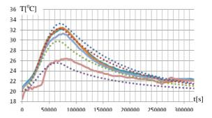
Figure 3: Comparison of the temperature characteristic for measured (solid lines) and indentified (dotted lines) of the temperature in sensor points.
