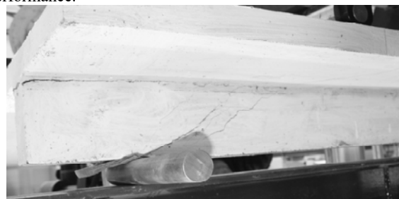
Figure 4: Example of crack pattern in the support zone of a BZ/S beam at the ultimate load.
